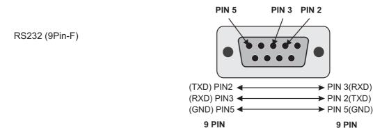
The wire must be changed between 2,3 pin.
