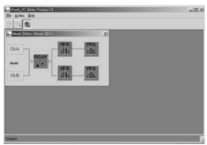
Select OPTION from the FILE menu, then select the right COM port (COM1 and COM2) and proper BOUDRATE (transmitting rate between this unit and your computer).
