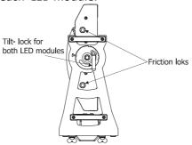
Danger of injury! Two workers have to handle with the fixture including adjusting the LED modules to the desired position. The LED modules are very heavy.
