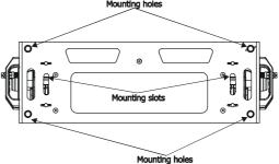
The mounting holes in the Omega holders have a diameter of 13 mm. Use the clamps with M12 bolts only. The four mounting holes in the fixture base have a diameter of 17 mm. Use M16 screws for fastening.
