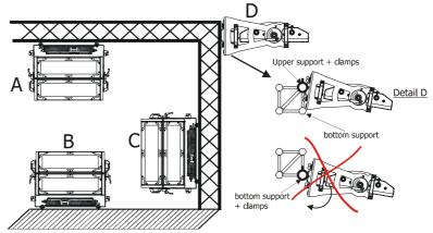
For securing of the fixture on a flat surface in the position **B** serves two mounting slots of diameter 8.5mm in the fixture base.
