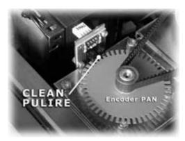
The sensors of the encoders concerning the PAN and TILT movements are located in the base and in the arm of the MP700 Zoom respectively. The pictures clearly show how you can reach these components and where you can correctly operate for their maintenance.
