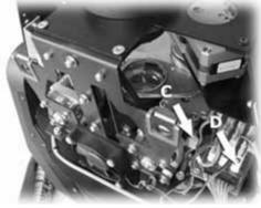
Once the frame with the Zoom/Focus mechanic unit has been removed, it is possible to clean the parts which are usually difficult to reach. Reassemble the Zoom/Focus unit carefully, being sure in particular that the blade with prism and frost is positioned between the two lenses of the Zoom/Focus unit. Remember then to connect again the 2 motors and the fan to their connectors.
