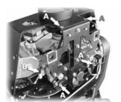
To make an extraordinary maintenance, it is necessary the presence of a generic or qualified mechanical operator, according to the type of the needed intervention. In order to make its use easier, we advise you to completely draw out the mechanic unit of the zoom and focus movements as follows: disconnect the two motors (connectors **B** and **C**) and the fan (connector **D**); remove the 4
