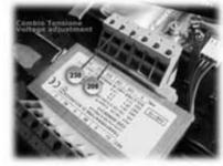
The fixture can work at the following tensions: 230 V~50 / 60 Hz and 208 V~ 60 Hz (optional). Please be careful to connect the cable to the right terminal that is relevant to the desired tension and frequency; both on the ballast and on the transformer located in the **MP700Zoom** base. Please carefully follow the indications shown in the pictures **A**
