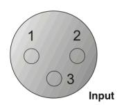
For unbalanced use PIN 1 and PIN 3 have to be bridged
