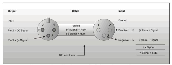
Compensation of interference with balanced connections
