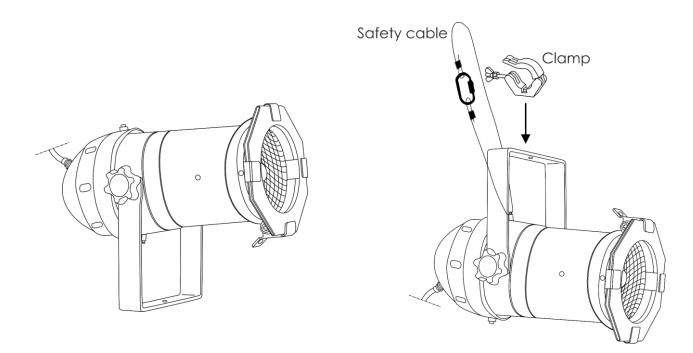
The PAR 46 Warm-On-Dim can be placed on a flat stage floor or mounted to any kind of truss by a clamp.
